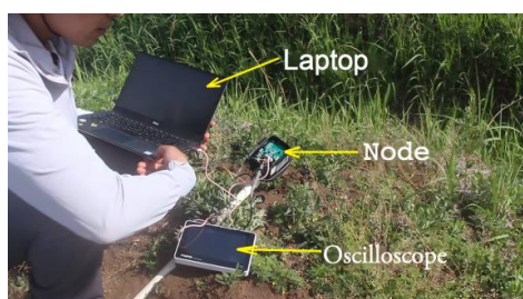
Figure 3: Field experimental operation of RS-485 interface
